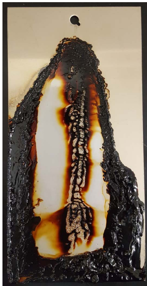
Closed Coke Pattern 90% Group III 10% AN-19
