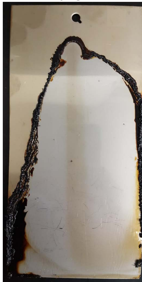
Open Coke Pattern Passed at 220°C
