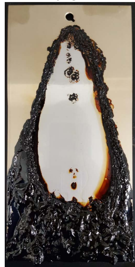
Closed Coke Pattern Failed at 230°C
